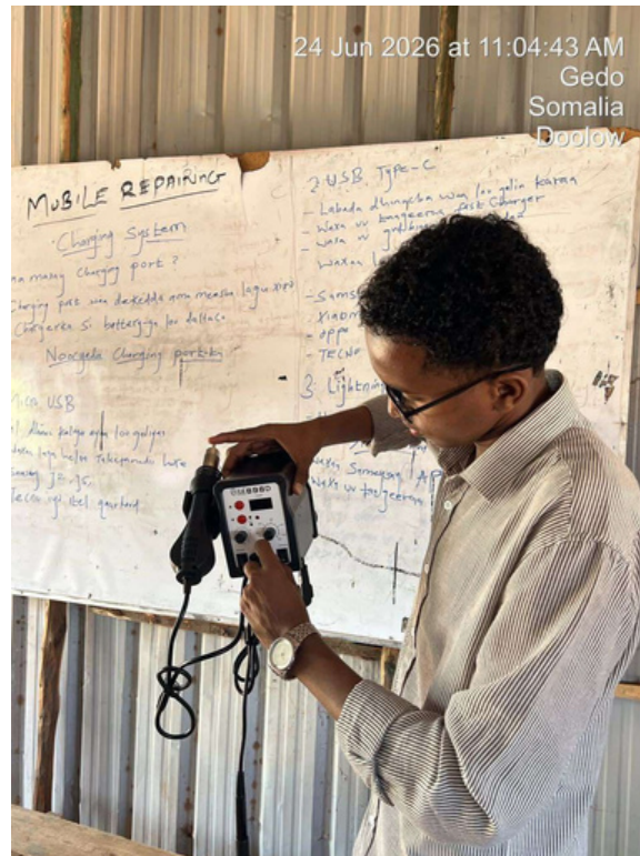
Trainer demonstrating use of a hot-air rework station, with charging-system notes on the whiteboard, 24 June 2026.
